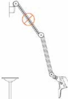
Arm under lower work area. Overload of arm.
