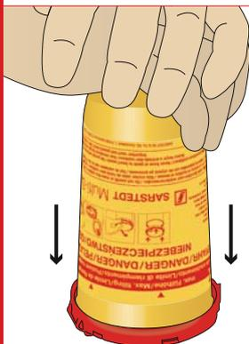
Put the lid on a stable surface and place the bottom part of the disposal box on the lid from above. Push the bottom part onto the lid so that the outer edge of the bottom part audibly and visually snap into place.
