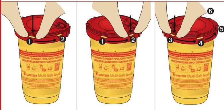
Centre the lid on top of the bottom part of the box. With your thumbs to the left and right of the gaps in the lid, push the lid onto the bottom part until the outer edge of the yellow bottom part audibly and visually snaps into place (1). Repeat this process for the remaining gaps in the lid (2–6).
